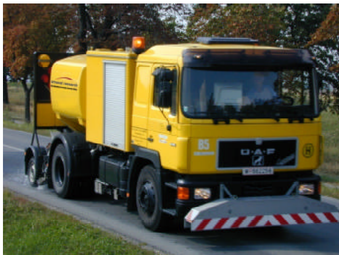
RoadSTAR (Road Surface Tester of Arsenal Research)
